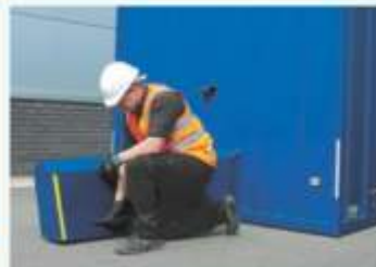
Close & lock canopy to protect towing facility
