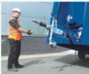
Unhitch from towing vehicle and operate hydraulics using the push button controls
